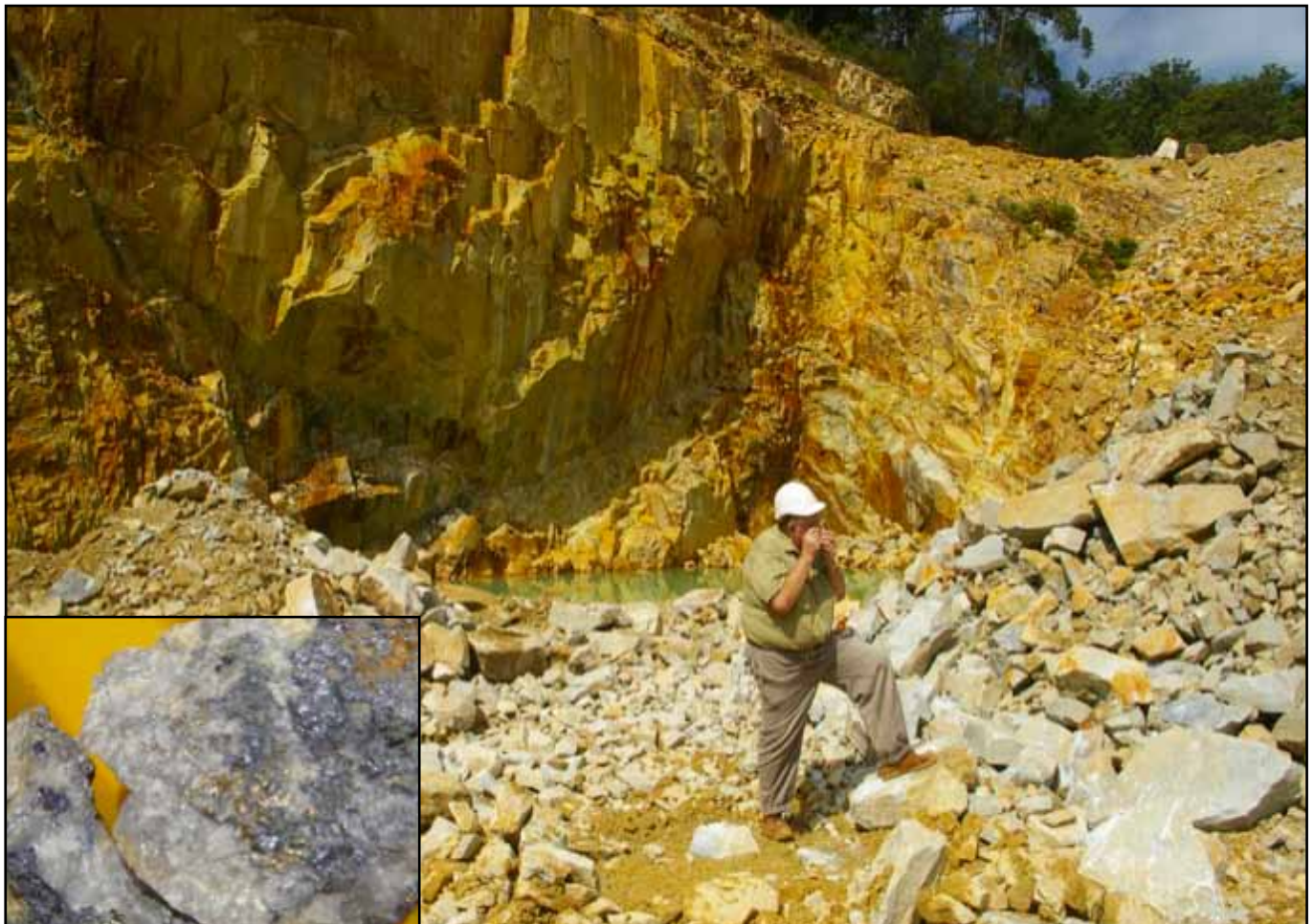
Figure 4 Valla Project showing Marriott’s quarry and high grade molybdenum mineralization (silvery grey mineral - inset)
