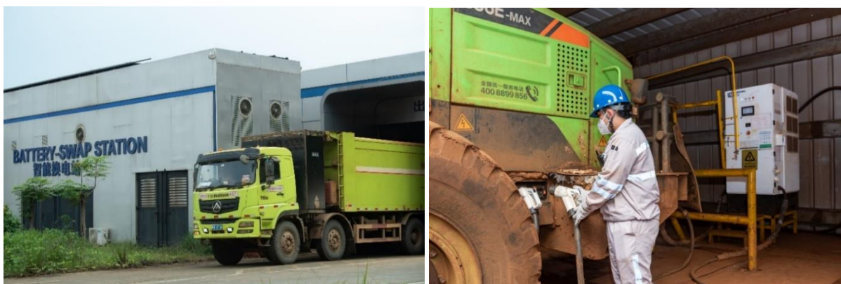
EV battery swap station and electric loader
