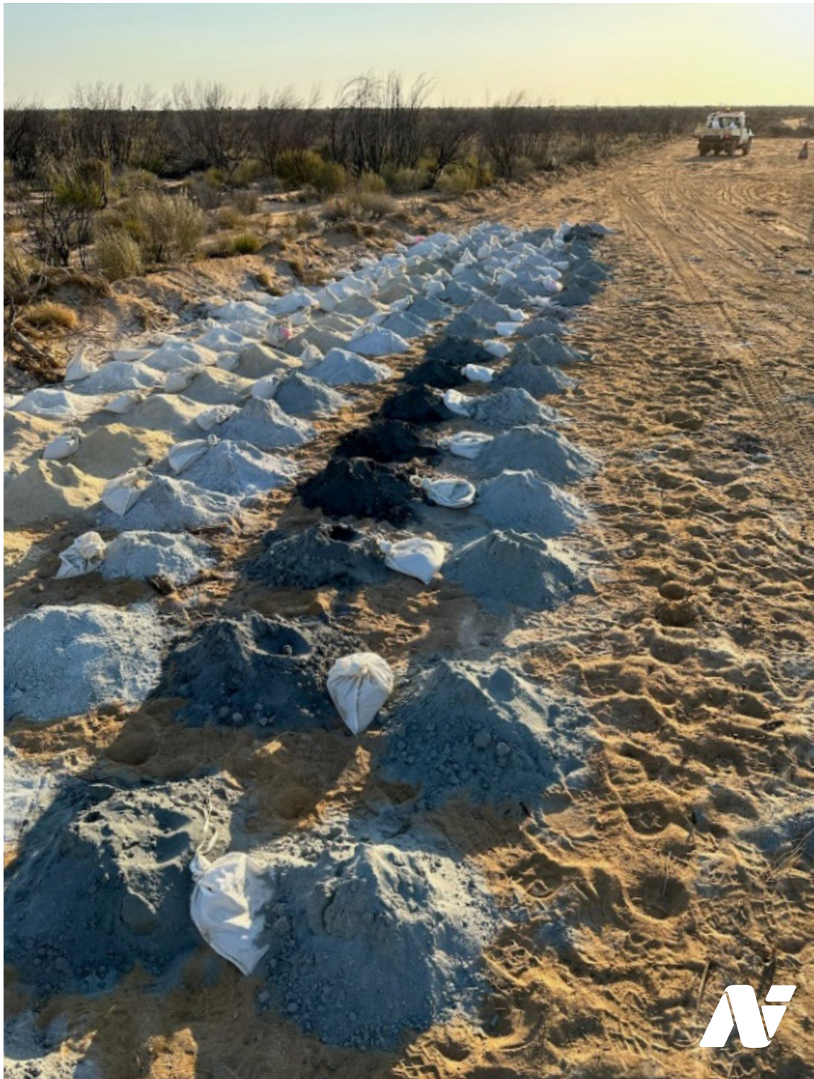
Figure 3 – 23NRRRC100 R/C Drill Piles, black material represents massive sulphide intersections.
