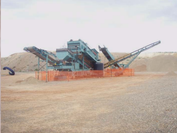
Mobile power screen unit processing local scats for various construction materials
