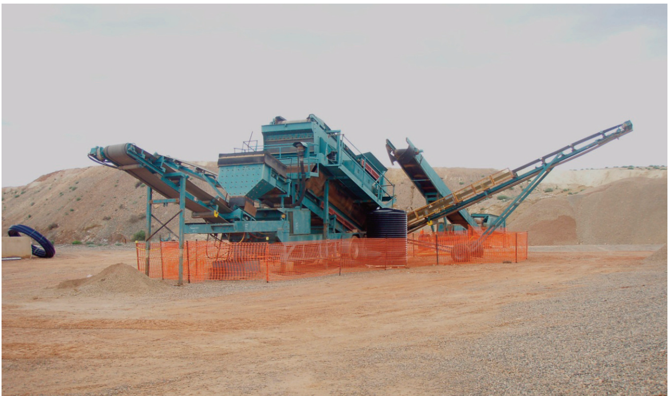
Photo 2. Power screen unit producing gravel for construction materials.
