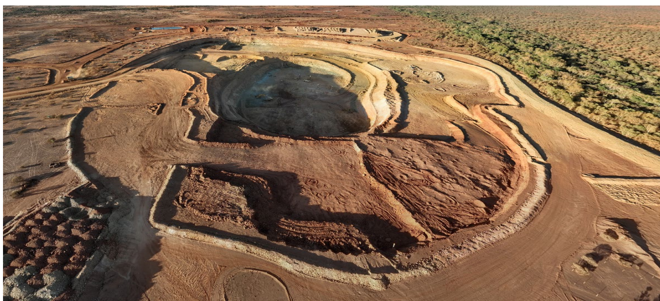
Progression of Stage 1 pit inside larger Stage 2 pit boundary
