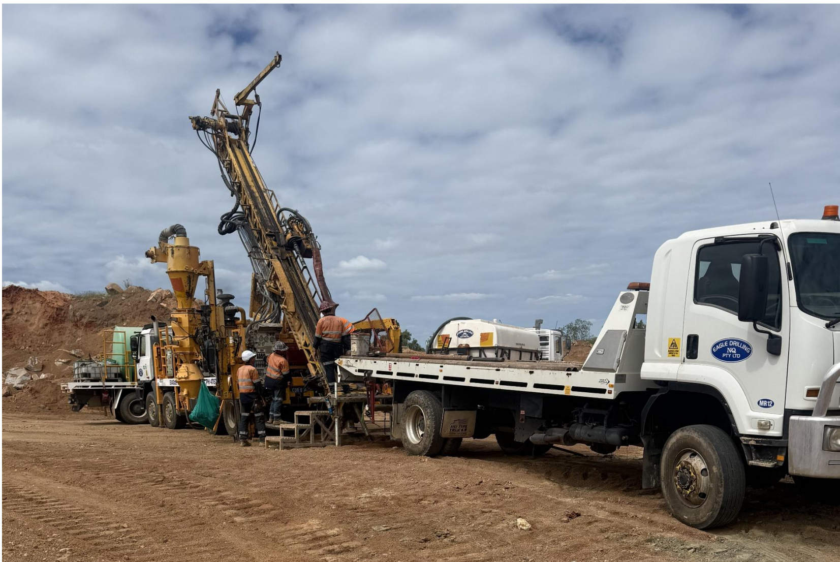
Figure 7: Diamond drilling North Central pit.
