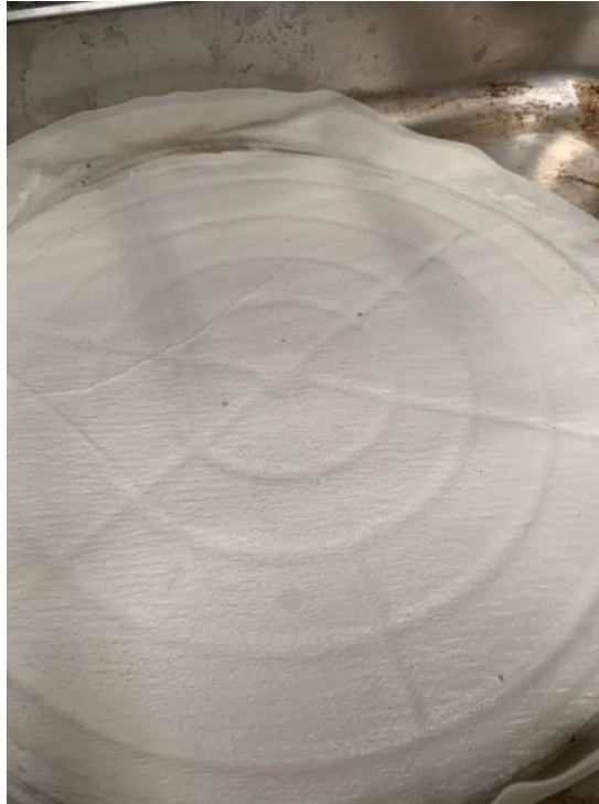
Figure 3 – Titanium hydrolysate production from bench test work on Barrambie leach residue
