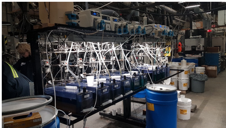
Figure 2 – Nickel Recovery Circuit of the Neometals Pilot at SGS
