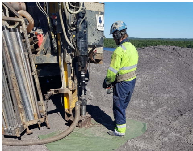
Figure 7: Metallurgical sample drill rig on Slag stockpile at SSAB Luleå
