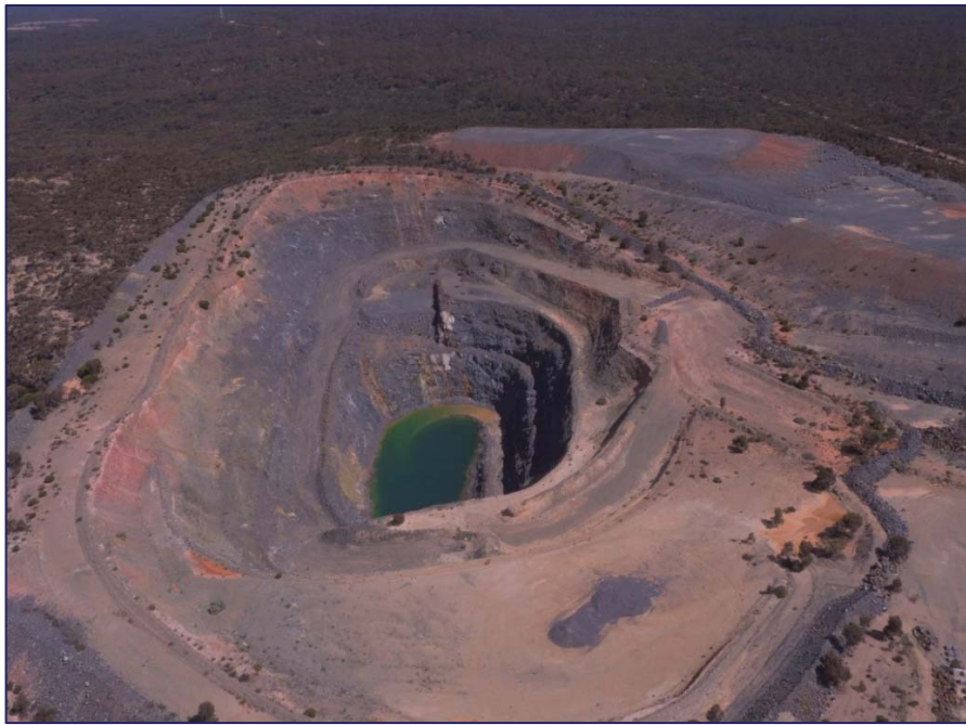
Figure 3 – View looking south over the 132N open pit. The 132N Mineral Resource continues beneath the pit plunging to the North at around 40°.
