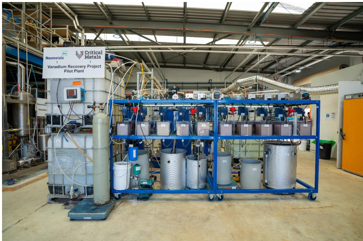
Figure 2 – Solvent Extraction section of Pilot Plant
