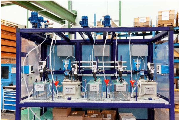
Figure 9 – Single Solvent Extraction Mixer/Settler Circuit
