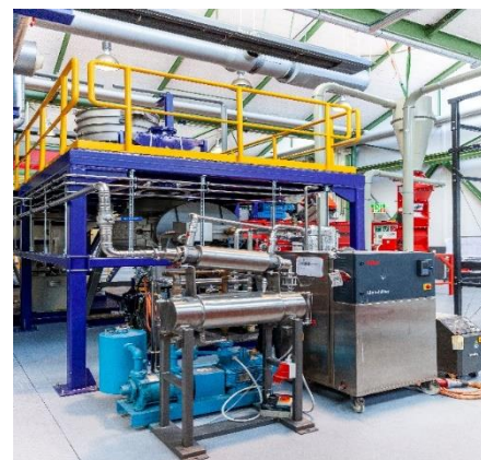
Figure 7 – Black Mass (Powder) Vacuum Dryer, Condenser and Electrolyte Recovery Circuit
