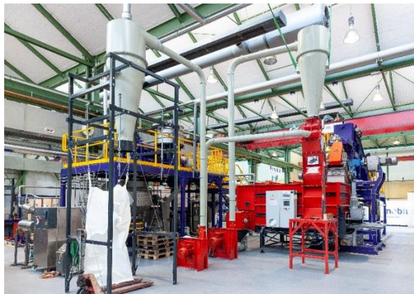
Figure 6 – Shredder feeding into – Primary Classification Circuit (foreground -red) removes and bags, plastics and Cu/Al metal
