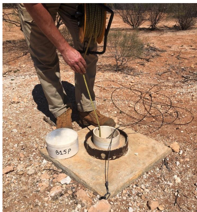
Figure 24– Dipping Production Bores at Barrambie
