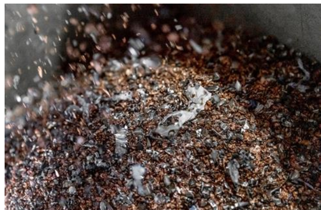
Figure 5 – Recovered Copper and Aluminium foil
