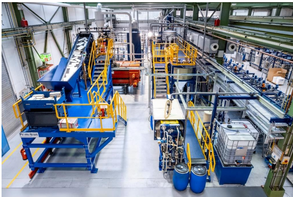
Figure 3 - Shredder and beneficiation processing EV cells
