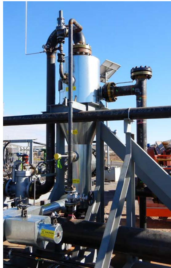
Knock Out Pot (a cyclone that collects and separates water and impurities from Syngas)
