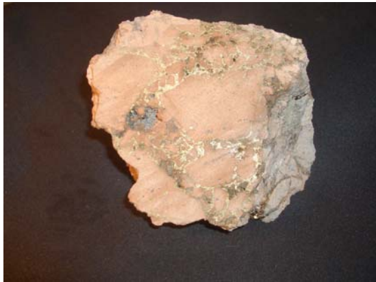
Redbank primary copper ore, pipe breccia with chalcopyrite matrix.
