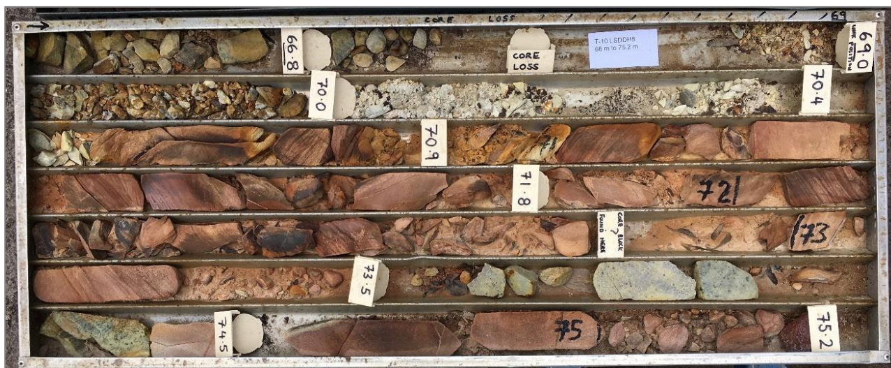
Figure 10.1 Example of poor DD core recovery as seen in hole LSDDH8 (Tray #10; 66.4–70.5 m)
