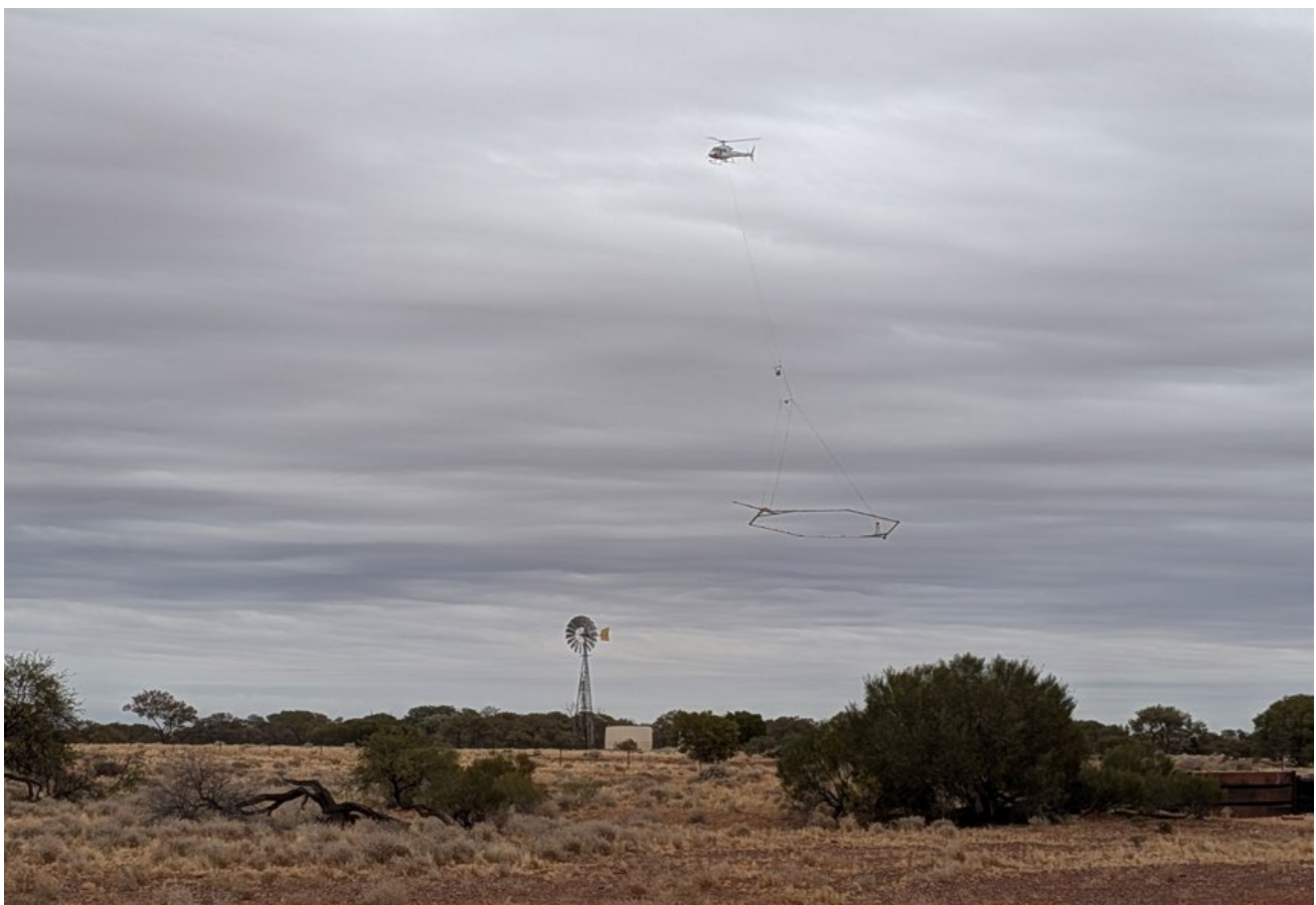
Figure 8 – Helicopter acquisition of high-resolution SkyTEM Airborne EM survey data over the Marymia East project.
