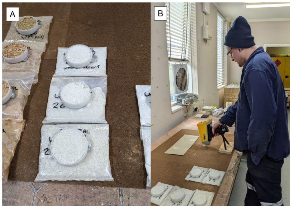
Figure 1. A) Historic aircore sample identified as saprolite / pallid zone from the bottom of hole. (Historic heavy mineral exploration drillhole by Red Metals Ltd, drilled in 2006). B) Portable XRF analysis by Challenger Geological Services, Adelaide
