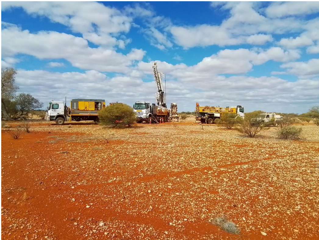
Figure 1: RC drilling of EM conductor in the Mt Nairn area, Narryer Project, WA
