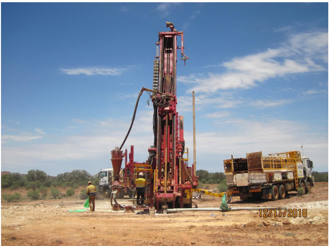
Plate 1 – TopDrill's 685 Schramm RC rig commences Musgrave drilling program for Woomera Mining Ltd
