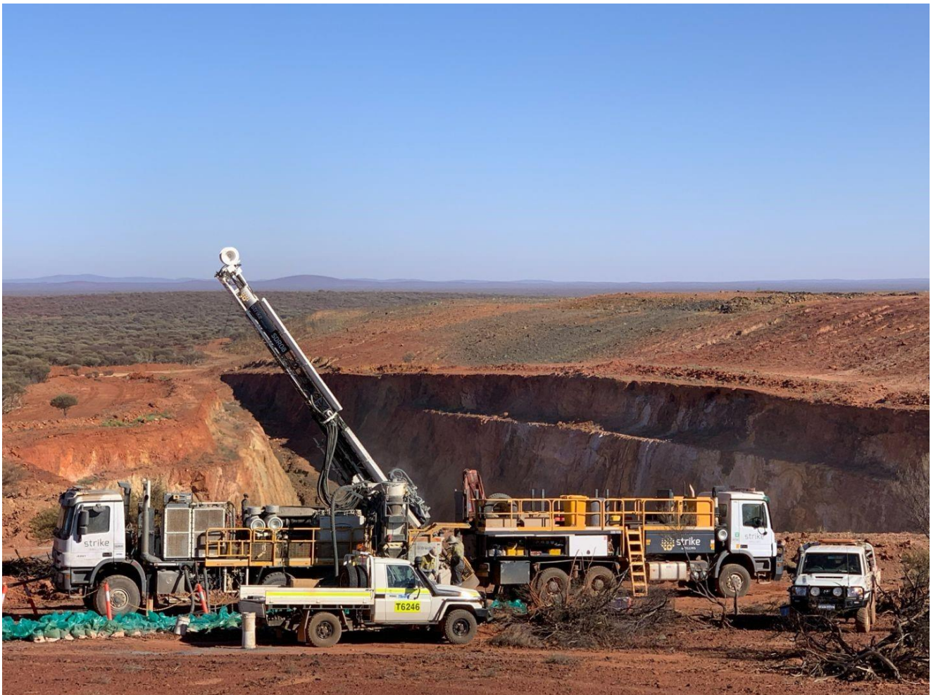
Figure 10. RC drilling activities underway at Bottle Dump.
