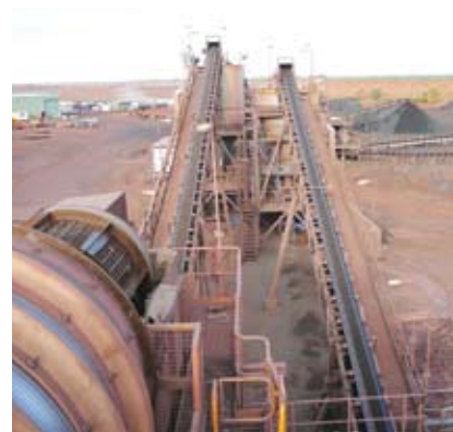
Product leaving the scrubber, lump on left and fines on right
