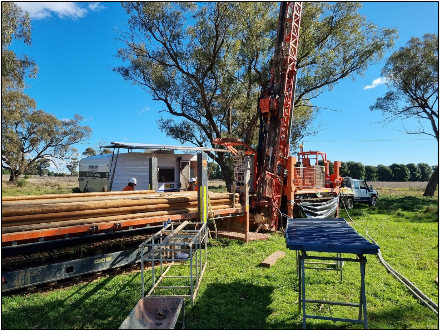
Figure 2 - Diamond drill rig set up on first hole (OCDD001)
