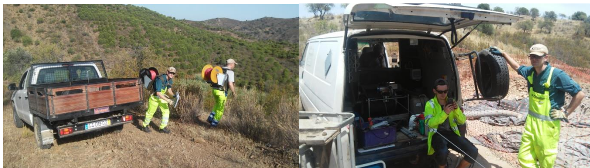
Figure 6 (a) Laying out surface cables for DHTEM reading.
