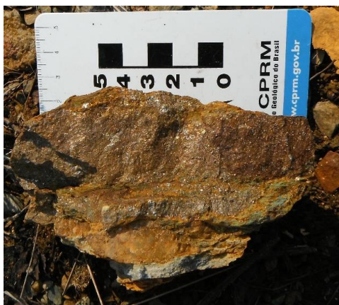
Figure 1. A. Massive sulphide sample collected from Tisová waste dump. Sulphides include; pyrite, pyrrhotite, chalcopyrite. B. Waste 1 at Tisová minesite
