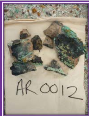
Shear zone with copper staining within Kanyaka open pit 12.40% Cu, 2.42% Zn & 0.47% Co.
