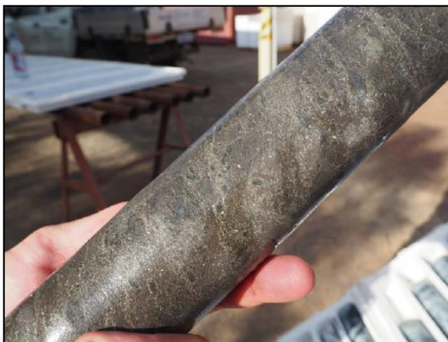
Photo 2 – 3: Massive pyrrhotite – pentlandite (nickel sulphide) – pyrite – chalcopyrite in drill-hole SNDD005 at Saint Patricks: 1.77m @ 6.72% Ni, 0.27% Cu and 0.13% Co from 227.31m down-hole.
