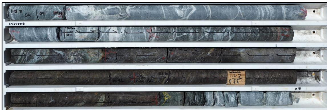
Photo 1: Massive pyrrhotite – pentlandite (nickel sulphide) – pyrite – chalcopyrite in drill-hole SNDD006 at Saint Patricks: 2.22m @ 4.84% Ni, 0.34% Cu and 0.15% Co from 110.68m down-hole.
