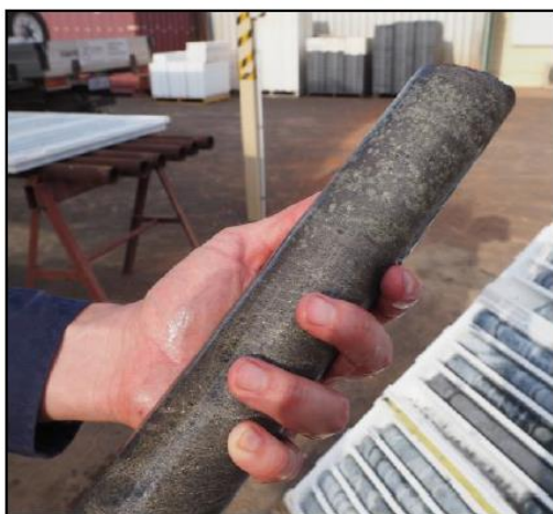
Photo 2 – 3: Massive pyrrhotite – pentlandite (nickel sulphide) – pyrite – chalcopyrite in drill-hole SNDD005 at Saint Patricks: 1.77m @ 6.72% Ni, 0.27% Cu and 0.13% Co from 227.31m down-hole.
