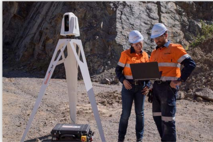
Geotech Monitoring Station (GMS) - laser-based monitoring solution
