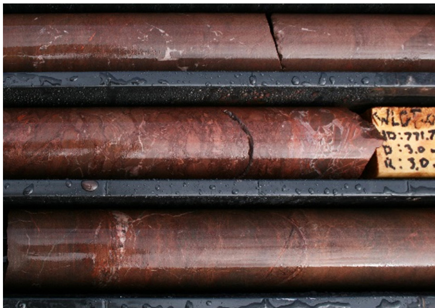
Photo 2 WLTD002, 770.5m to 772.7m, Murdie Project: IOCG-style hematite alteration and brecciation.
