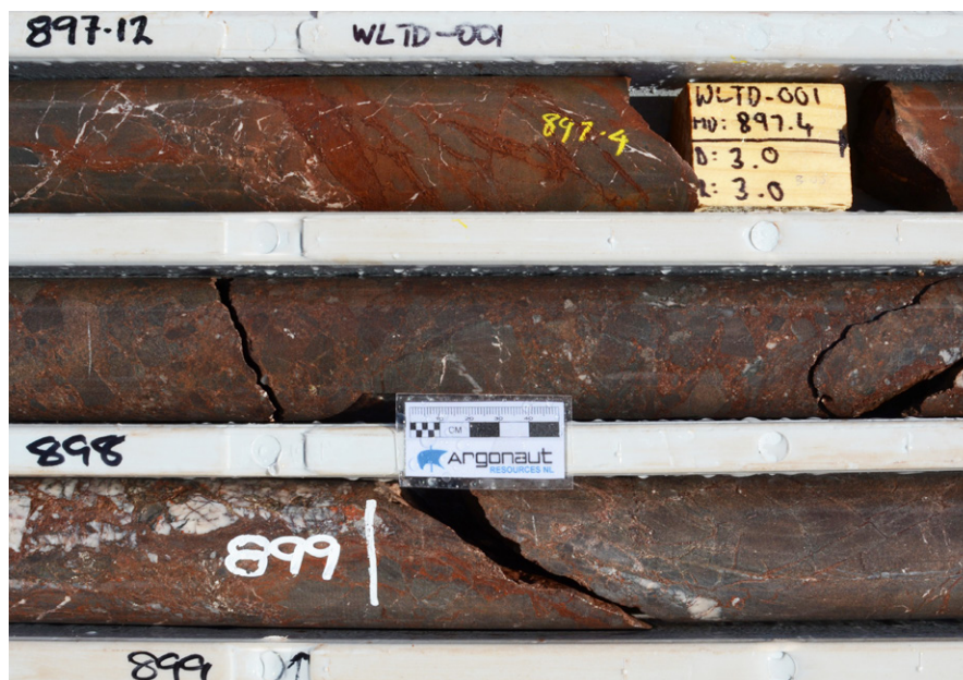
Photo 1 WLTD001, 897m to 899m, Murdie Project: IOCG-style hematite alteration and brecciation.
