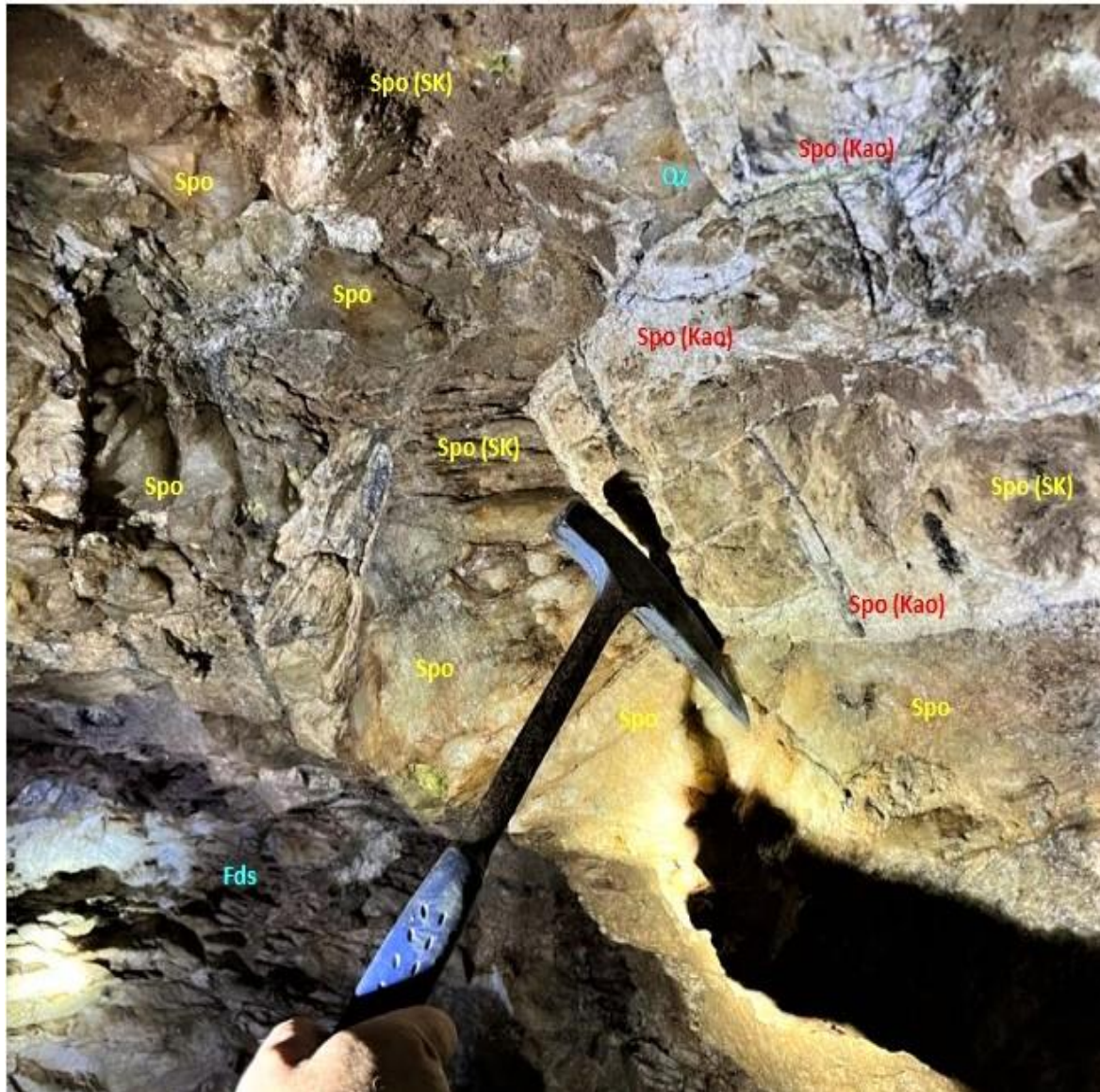
Figure 6: Typical of spodumene crystals within Spodumene Zone in Jaime Linopolis Sitio do Estevinho underground mine. Massive fresh spodumene (Spo) . White domains are partially kaolinized spodumene along fractures (Spo Kao). Spodumene with skeletal/corroded texture (Spo SK). Spodumene occupies at least 60% of the field of view in this picture.
