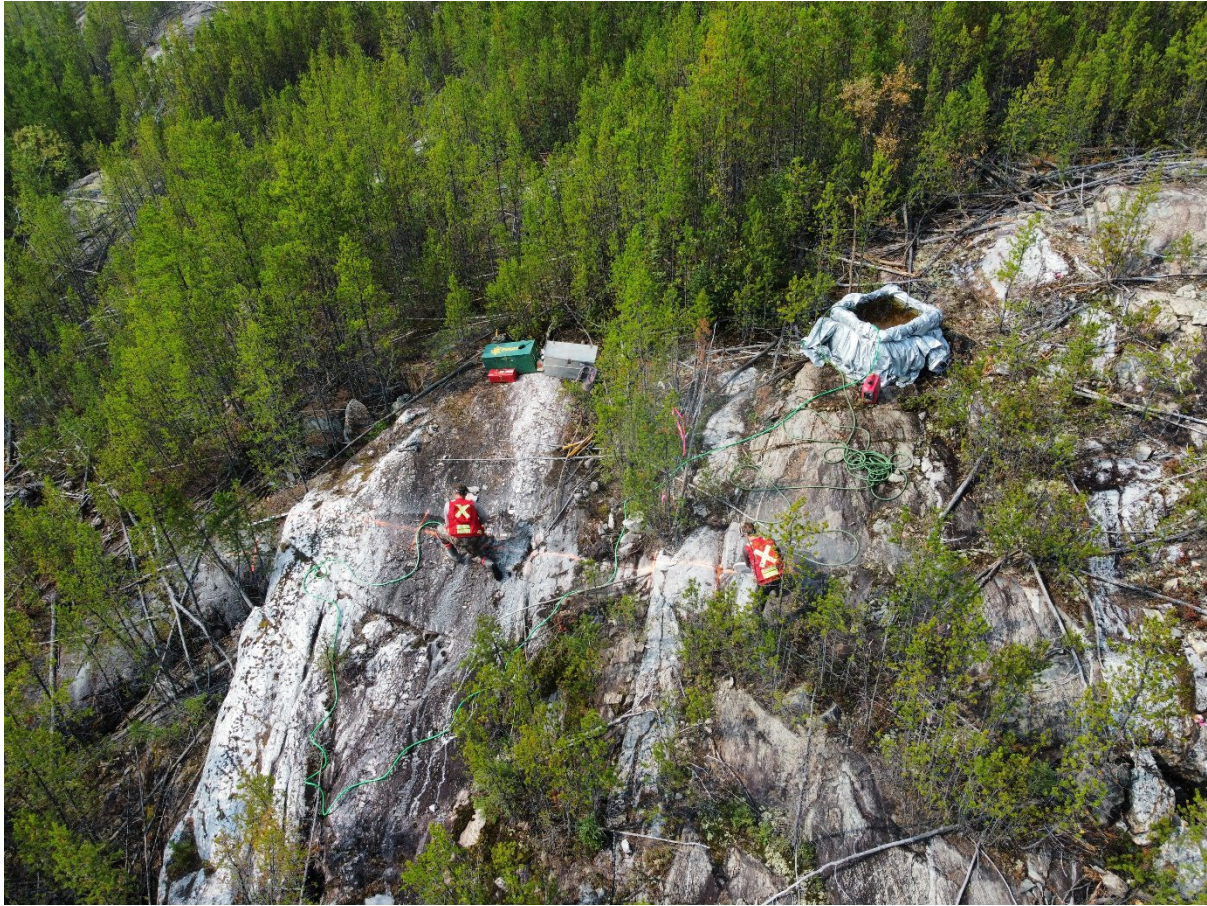
Figure 2: Channel sampling across an outcrop of the G2 pegmatite at Gorman. See Figure 5 for detail.
