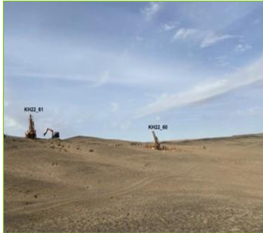
Two core rigs drilling from surface down to 200 metres with team from Temarise and SRK on site
