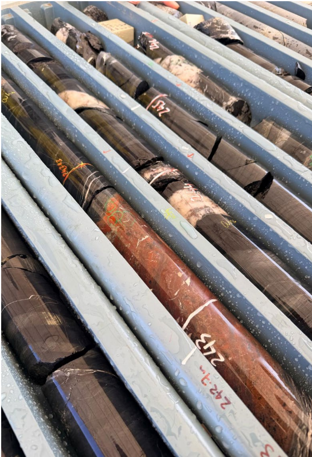
Plate 5 - SDH25-032, illustrating the sheeted veining mineralisation surrounding the recently discovered Hematite-magnetite matrix zone in Macau
