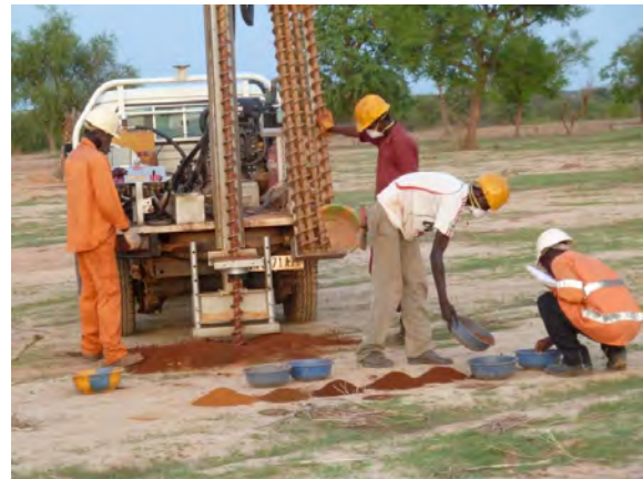
Power auger drilling, Laterite Hill Gold Field, Burkina Faso
