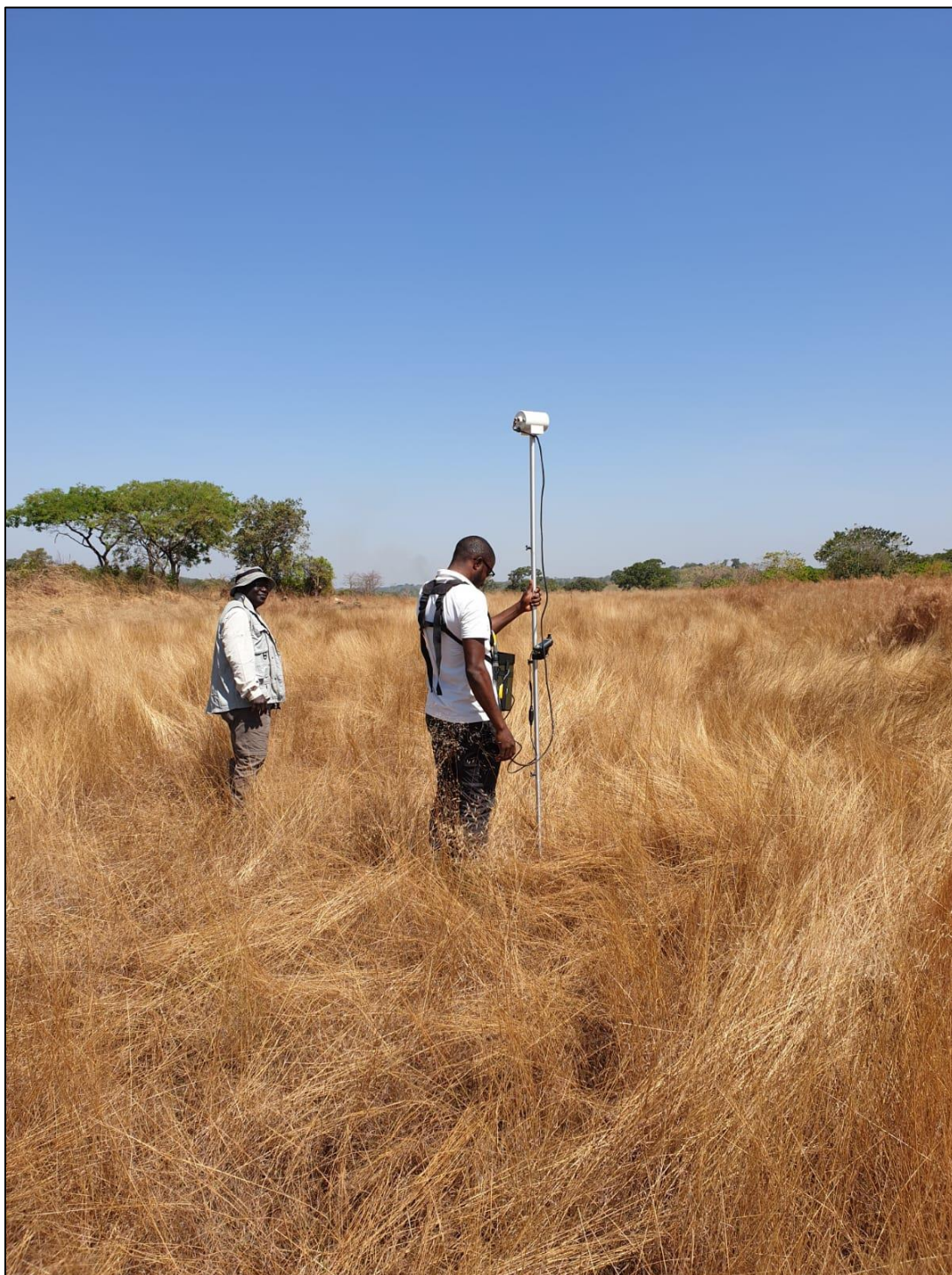
Figure 4 - Predictive Discovery Principal Geologist Aimé Nganare (left) supervising ground magnetics survey on the Kankan Project.
