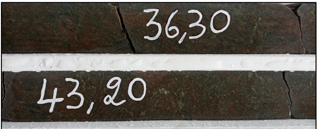
Figure 4 - Representative high grade drill core from hole BNEDD0088 (324-326m) – intense pink feldspar alteration of tonalite with abundant pyrite (iron sulphide) veins. 1m gold grades are shown as annotations on the core.
