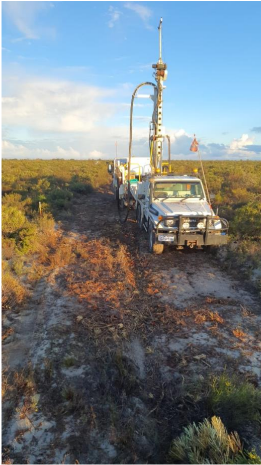
Images 2 & 3 – Air-core drill rig set up for drilling (left) and white sand horizons being encountered (right) during June 2021 drill program
