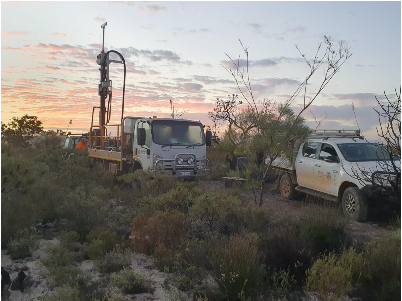
Image 1 – Air-core drill rig and support vehicle in the field during the June 2021 drilling program
