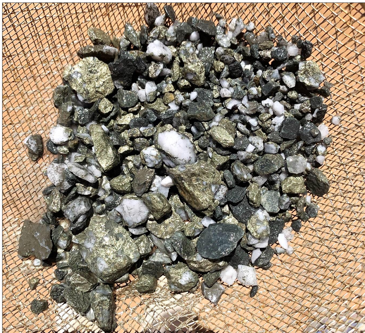
Figure 1: WLRC069 - 259m: Semi-massive chalcopyrite + quartz veining + chlorite-altered volcanics/seds
