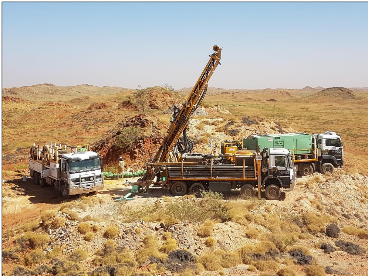
Figure 1: Reverse Circulation (RC) drill rig at the Old Faithful deposit, Mt York Project.
