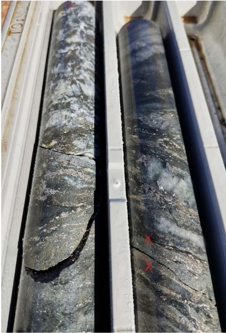
Photo 3: Typical higher-grade gold mineralisation at Main Hill from drill hole 25MYDD012. The NQ core (diameter 47.6mm for scale) is from 274-276m and is part of the intercept of 7m @ 2.66g/t Au. Left-hand core is 274-275m with grade of 4.12 g/t Au and the right-hand core is from 275-276m with grade of 2.9 g/t Au. Mineralisation within the BIF comprises quartz veining with associated pyrrhotite and arsenopyrite. Arsenopyrite is a key indicator of gold mineralisation. Note that extensive metallurgical test work indicates that mineralisation at Mt York is free-milling (see KAI ASX announcement dated 27 November 2024 entitled 'Strong Scoping Study forecasts robust financial returns').
