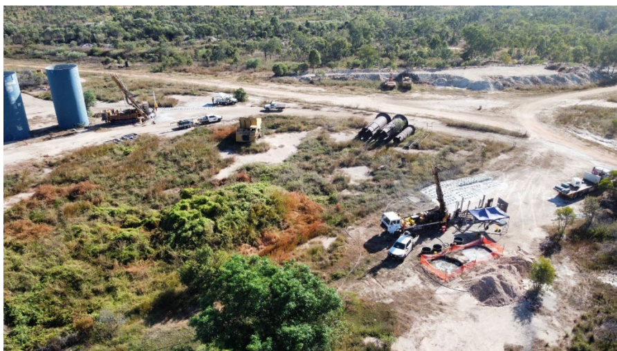
Figure 3: RC rig drilling top left and diamond rig drilling bottom right in photo targeting F1a high-grade zone
