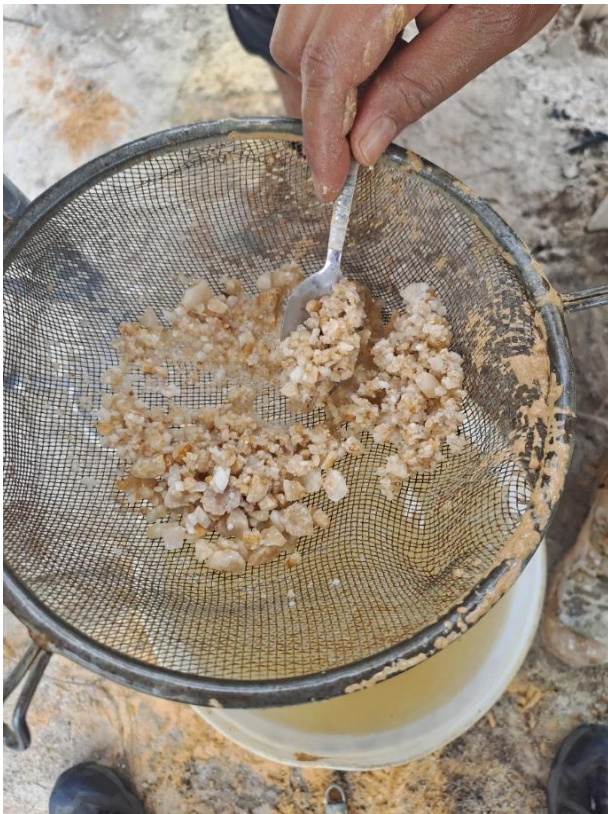
Figure 4: Chip samples from RC drilling, showing quartz veining in granite
