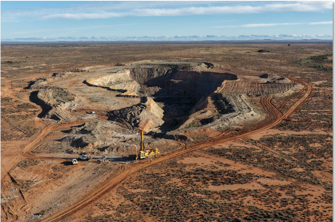
Photo 2: Photo of the RC drill rig operating at the Vertigo deposit, White Dam Gold Project, SA.
