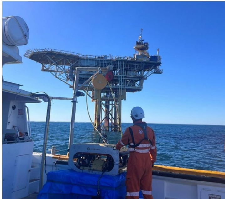
Photo 1: ROV being deployed off operations support vessel at Cliff Head Wellhead Platform
