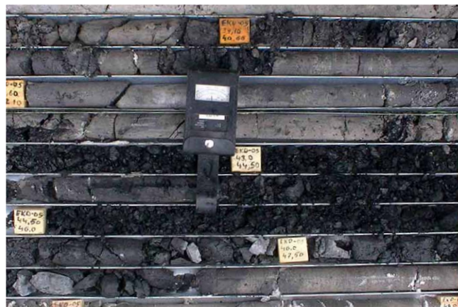
FIGURE 5 Uranium mineralisation in drill core from drill hole EKD 5
