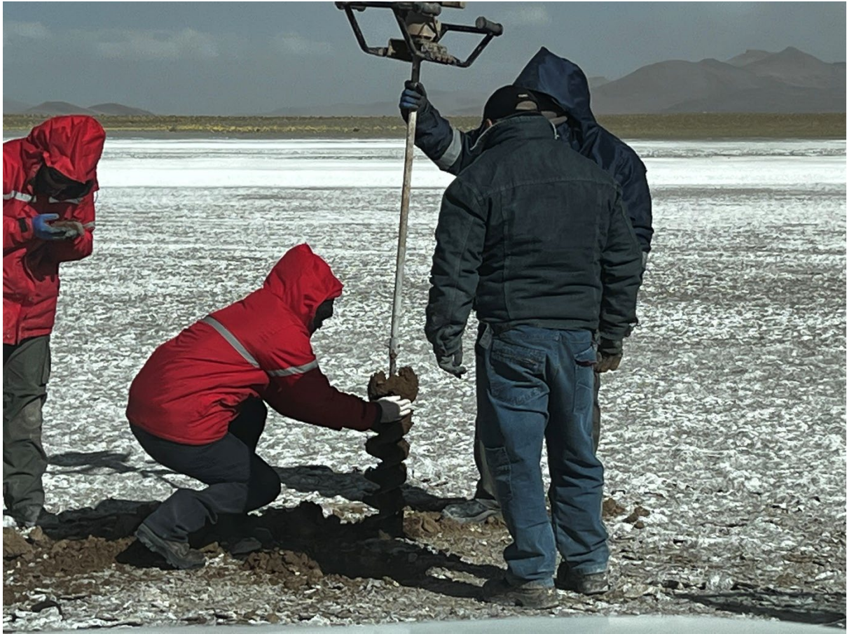
Figure 2. Technical support team operating motorised augur, and geologists examining soils and collecting black porous sands from augur for analysis.
