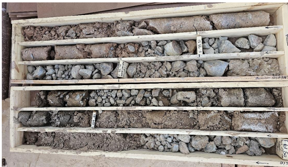
Figure 2. Core tray showing unconsolidated sands and gravels at 98m depth.
